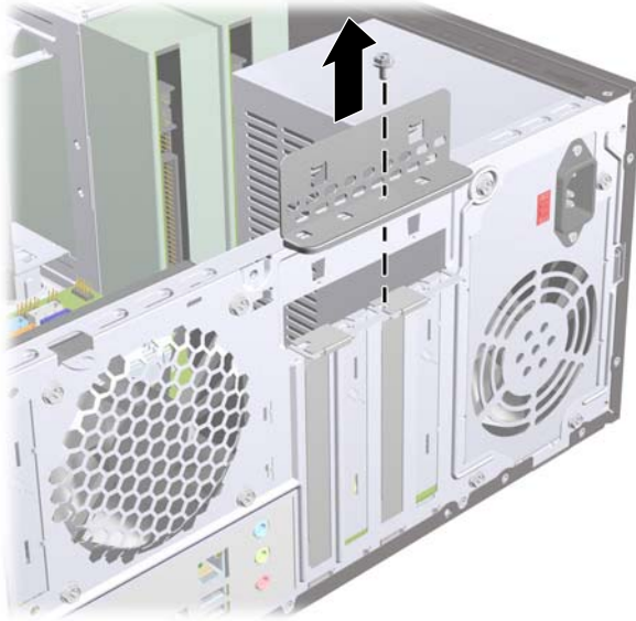
Figure 6-8 Opening the Slot Cover Lock
